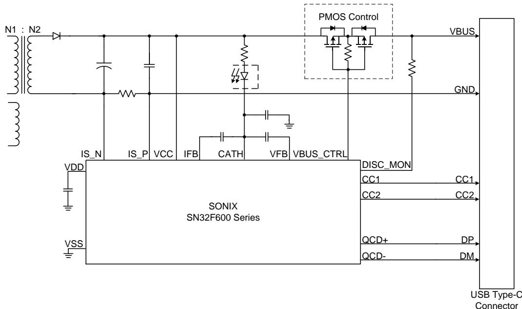
Figure 4–1 Power Adapter Application with PMOS Control
