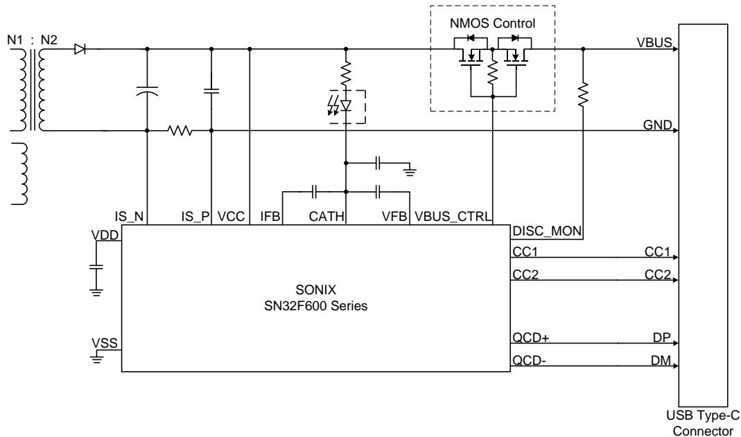
**Figure 4–2 Power Adapter Application with NMOS Control**
